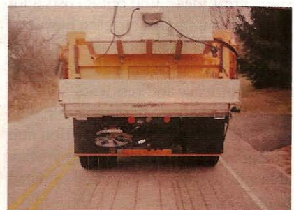
The anti-ice system designed and built using a 75-gallon pre-wet system manufactured by Monroe Truck Equipment.
