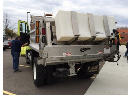
An example of a prewetting tank is shown above. This tank holds liquid deicer which is added to the granular deicer as it leaves the truck.
