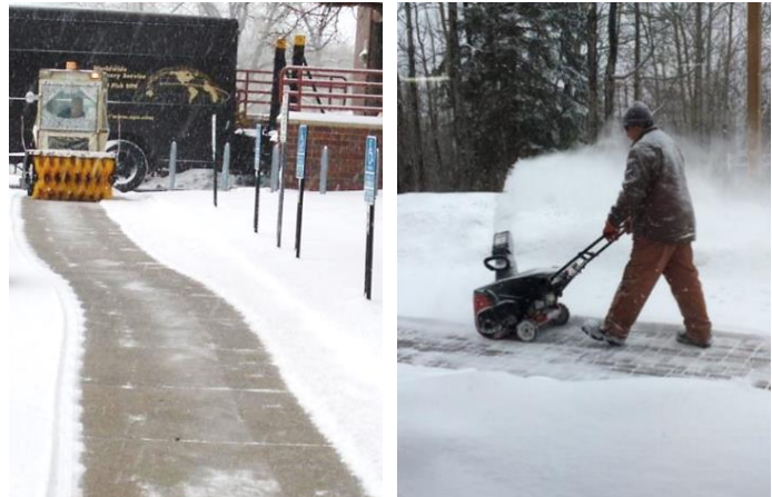
Brooms (left) remove snow closer to the pavement than most other tools (right).
