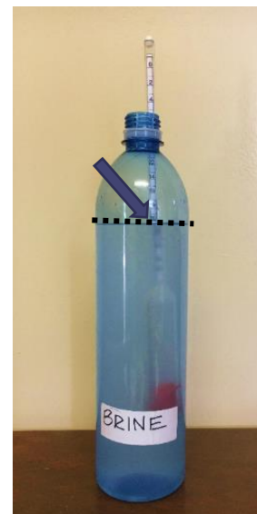
The photo above shows where to read a hydrometer to determine concentration. (marked by the arrow and dotted line)
