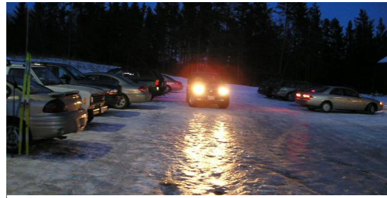
Icy compaction, such as the parking lot in this photo, can possibly be avoided with early mechanical removal.
