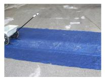
Lay down the tarp and measure out a 10-foot long stretch (hint: use tape on the tarp so you can easily see the 10-foot area). A longer test area can be used. The longer the test area, the more accurate the results will be. If a longer test area is used you will need to adjust this in the table on the back of this sheet.
