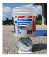
Sweep up and weigh the material that is within the marked 10-foot stretch.
